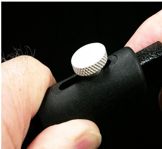
Make certain the screw is well tightened. The extra grip the screw threads provide when grasping the sides of the delrin slot (illustrated) don't seem like much but really do anchor the Extension Arm much more firmly in place.
