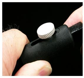
Make certain the screw is well tightened. The extra grip the screw threads provide when grasping the sides of the delrin slot (illustrated) don't seem like much but really do anchor the Extension Arm much more firmly in place.
